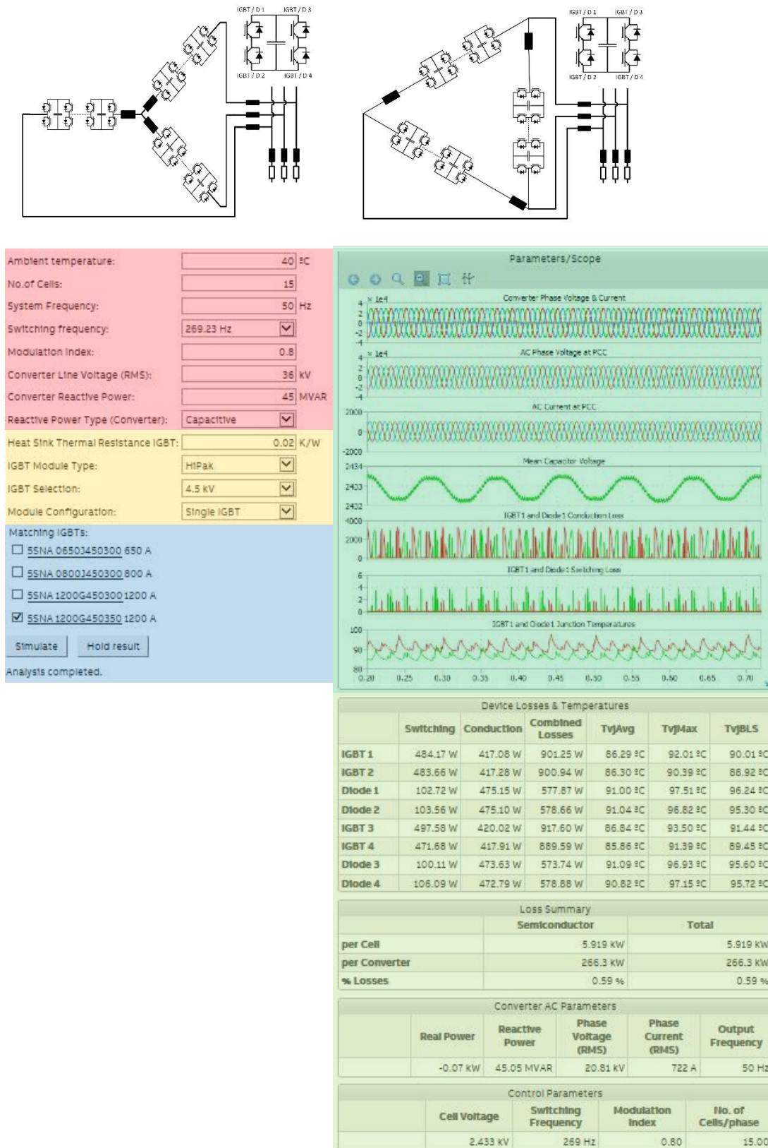
Figure 1 FACTS Full Bridge MMC with IGBT circuit on website
